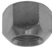
GL-0017 Hex: 13/16" Height: 5/8" Degree: 90 Plating: Zinc
