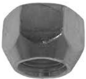
GL-0031 Hex: 13/16" Height: 5/8" Degree: 60 Plating: Zinc
