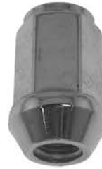
GL-0505 Hex: 13/16" Height: 1.4" Degree: 60 Plating: Chrome Bulge
