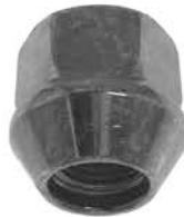
GL-0093 Hex: 13/16" Height: 59/64" Degree: 60 Plating: Zinc
