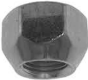
GL-0016 Hex: 13/16" Height: 5/8" Degree: 60 Plating: Zinc
