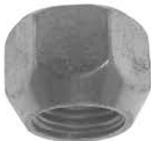
GL-0309 Hex: 21mm Height: 16mm Degree: 60 Plating: Zinc
