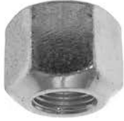
GL-0014 Hex: 3/4" Height: 9/16" Degree: 60 Plating: Zinc
